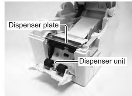
3. Peel off the first two leading labels from the liner (backing paper) and then pull out the leading liner (backing paper) from the **media holder**. Pass the liner (backing paper) over the **dispenser plate** so as to cover it. Then pass the liner (backing paper) under the **pressure bracket** as shown.
