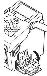
2. Insert the battery pack, then close the battery cover. Insert the battery pack with the connector side toward the printer.
