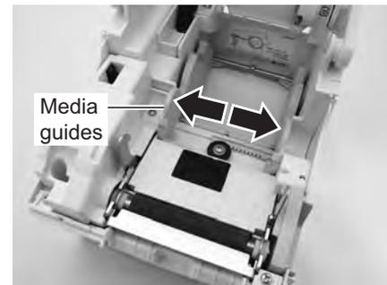
3. Load the media onto the **media compartment**. Then adjust the **media guides** inward till the **media guides** press lightly against the media roll. Turn the media roll lightly by hand and confirm that it rotates smoothly. Otherwise, media may not be fed correctly during operation.
