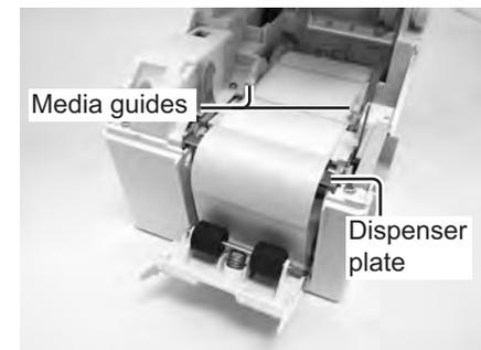
4. If the paper is not taut, roll the paper on the **media holder** so that the paper is taut. Next, tightly close the **pressure bracket** with the liner (backing paper) passing through it.
