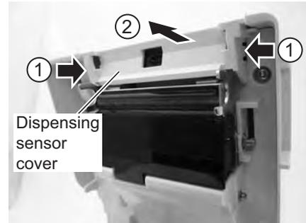
4. Press and push up the **print head assembly** to release it from the catches.
