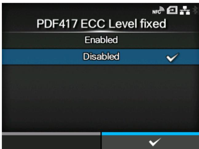
Set whether to print the PDF417 code with the security level specified by the PDF417 printing command.
