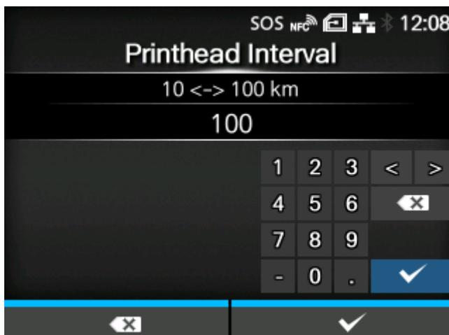
Set the notification interval about when the print head needs to be replaced.
