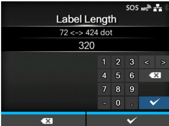
Set the label length manually when the [Micro Label Print Mode] is set to [Enabled] and the [Auto Label Length Detection] is set to [Disabled].
