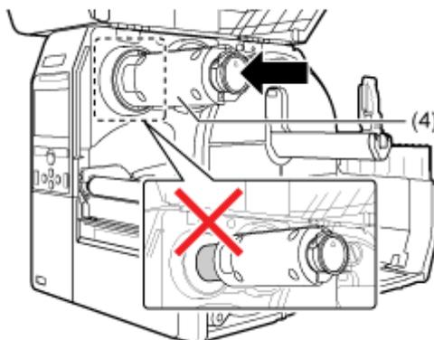
6. Remove the used ribbon core from the ribbon supply spindle.
