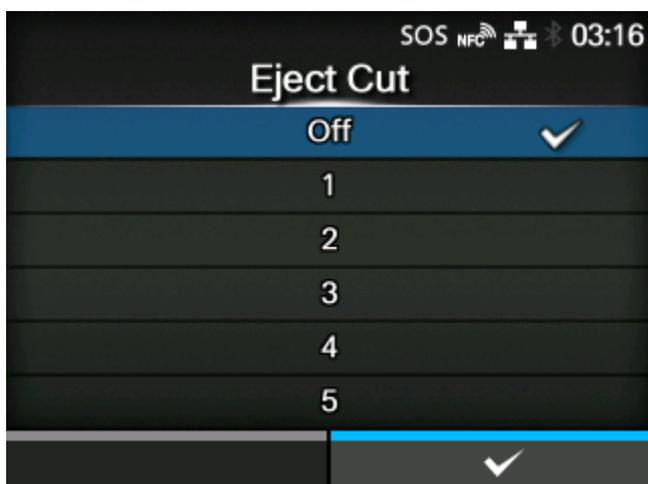
Set the Eject cut motion for the last printed media. Cut the last media after the specified timing.
