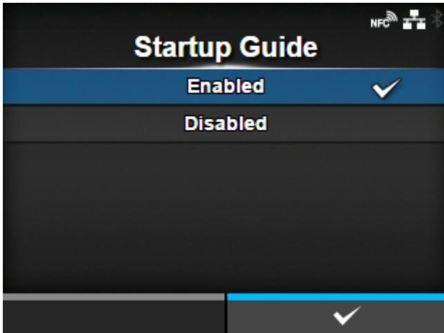
The startup guide is a function to help you through the initial product settings (such as setting date and time, and loading the ribbon and media).
