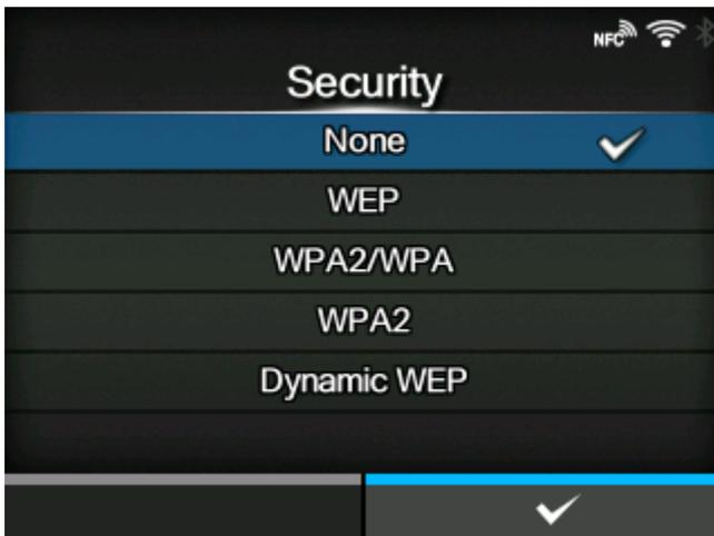
Set the security method of the network. Set the security methods so that the product, host and network devices match.
