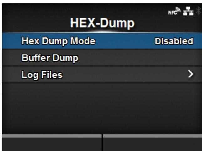
Save the hex dump print data or dump data from the receive buffer to the USB memory.
