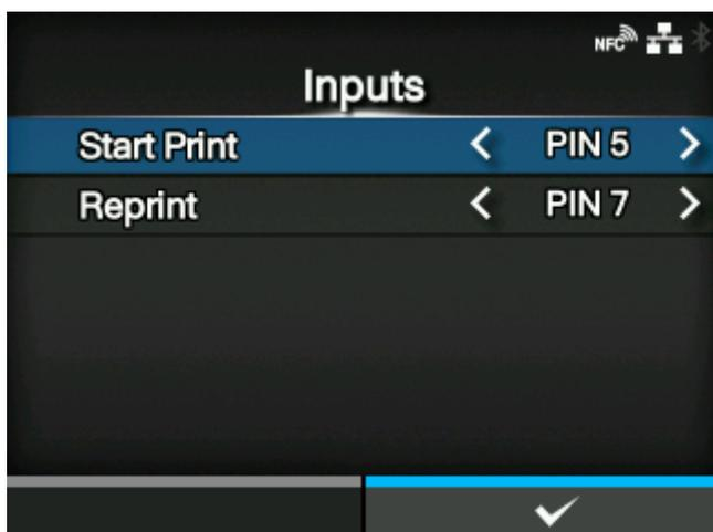
Assign the pin No. to the input signals Print Start and Reprint.
