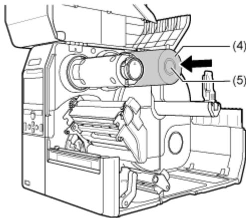
**5. From the ribbon supply spindle (5), pass the ribbon below the print head (6).**
