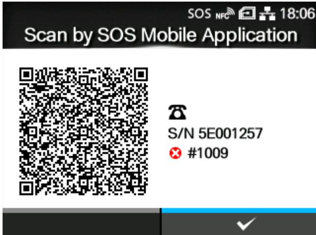
The menu for the specialized application for SOS appears after scanning the QR code with a tablet device or smartphone. NFC connection can be used for Android device to acquire the product's information. A specialized SOS application is required to scan the QR code or acquire the product's information with NFC connection.
