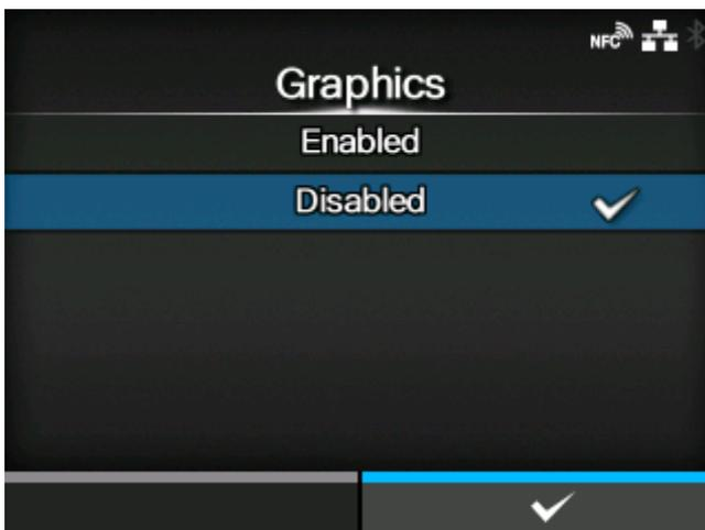
Set whether to allow the registration of graphic data even if a line feed code is omitted.
