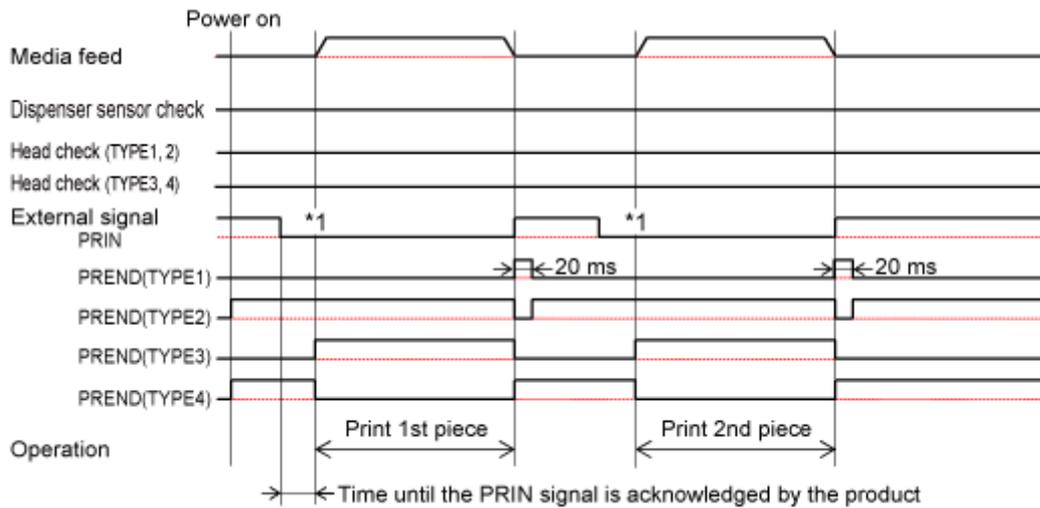
\*1 Keep the PRIN signal until the PREND signal is outputted.
