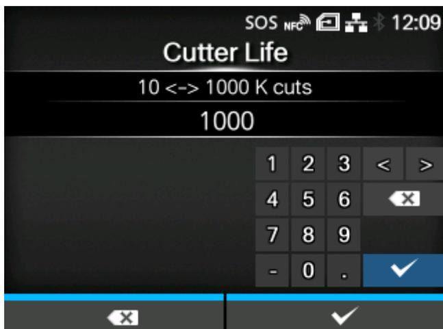
Set the notification interval about when the cutter unit needs to be replaced.
