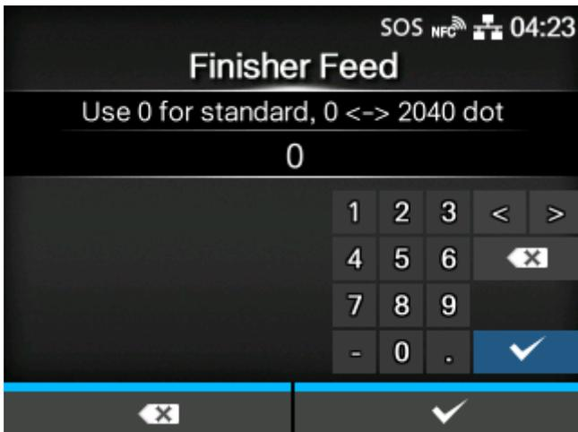
Set the media feed amount for Tear-off, cut and dispense stop. Set the media feed amount based on the print head position of 0.
