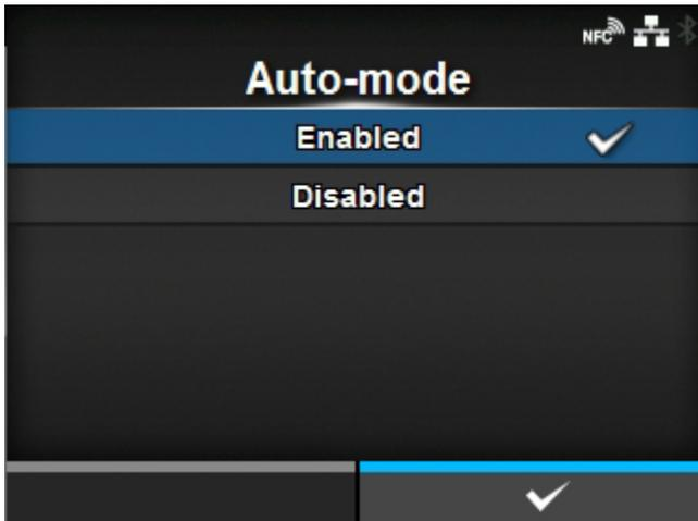
When using [Auto-mode], the print mode changes automatically according to the status of the installed option unit.
