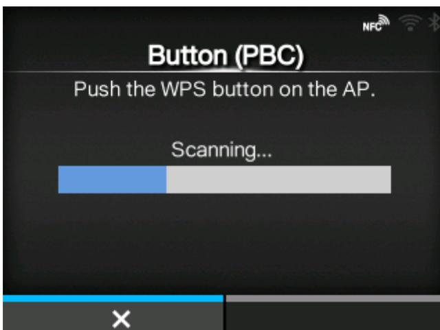
Set the wireless LAN connection using the push button method.
