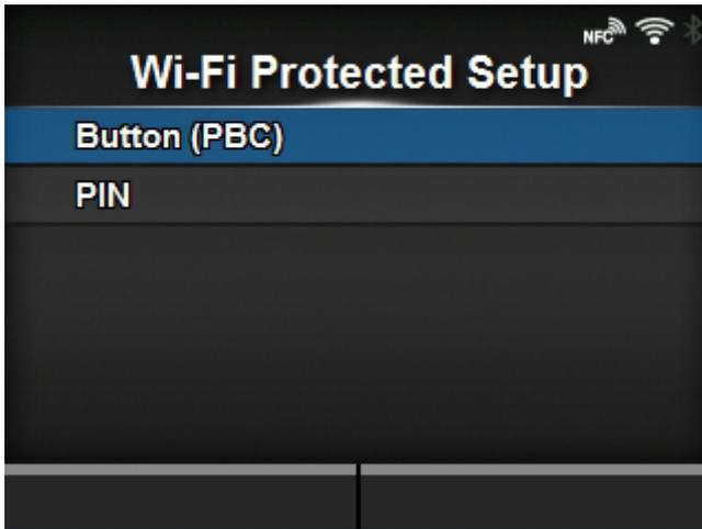
Set the wireless LAN connection using the push button or PIN code method.
