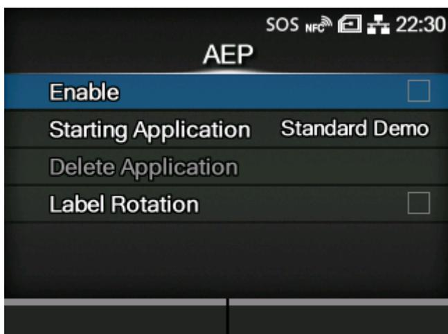
Set the functions for AEP (Application Enabled Printing).
