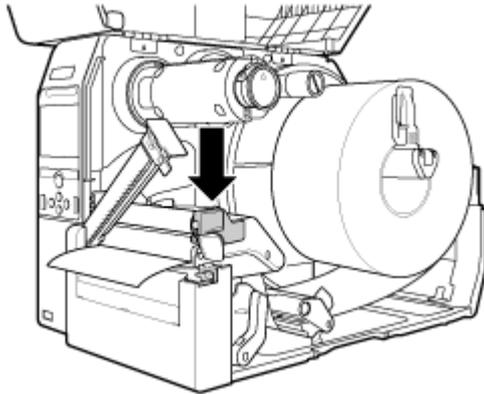
8. Close the cutter and then push the tab (7) in the reverse direction to lock it.
