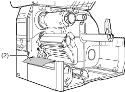
6. Press the print head down until you lock the head lock lever in place.
