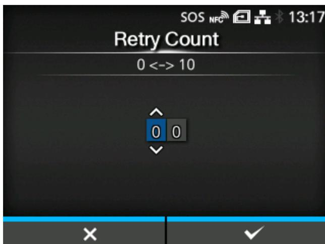
Set how many times the product will try to print and check the same barcode after VOID printing when a barcode reading error or barcode comparison error occurs.
