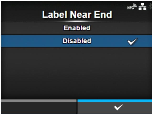
Shows or does not show the warning icon when the media is about to run out. Printing does not stop even if the warning icon shows up.
