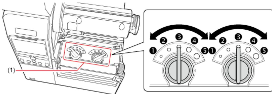
3. Turn the adjustment dials (1) according to the media thickness and set the head pressure.
