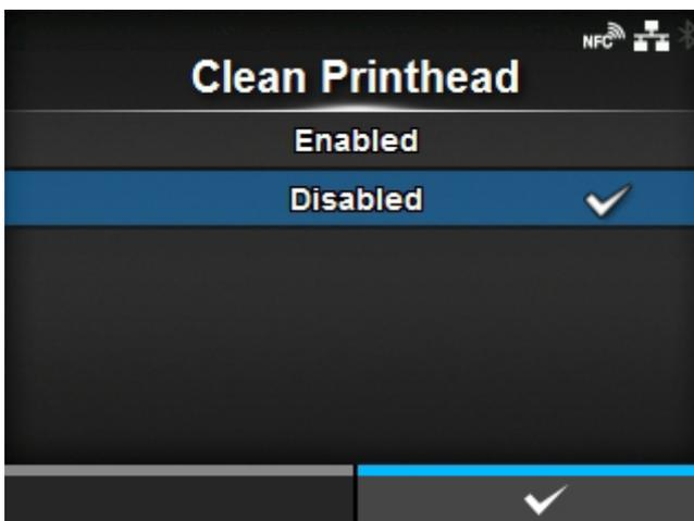
Enable or disable the notification function about when the print head needs to be cleaned.
