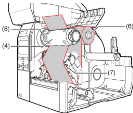
**9. Wind the ribbon counterclockwise to the ribbon rewind spindle (4) and grip sheet (8).**
