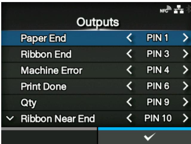
Assign the pin No. to output signals.
