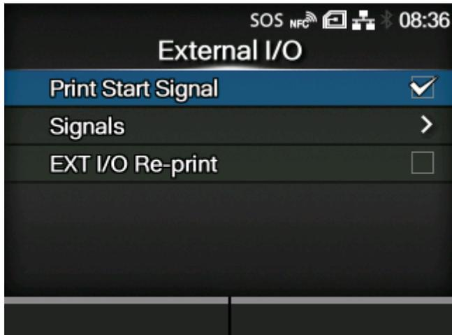
Use the external (EXT) terminal as an interface between the external device and the product.
