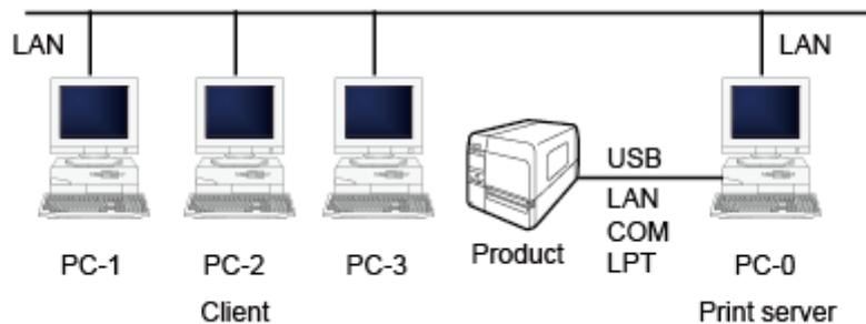
Set one computer (PC-0) as the print server and set other computers (PC-1, PC-2, PC-3, and so on) as clients. All computers should be connected using a LAN connection and the print server and product should be connected using LPT, COM, USB, or LAN.
