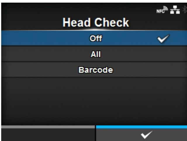
Automatically check if there is a broken element of the print head.
