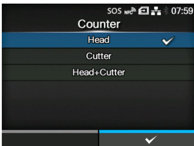
You can select the counter for the print head, cutter, or both for the timing to perform the periodic notification.
