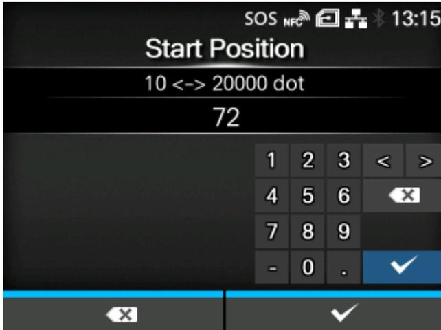
Adjust the position at which the barcode check starts (position of the barcode checker at which reading starts).
