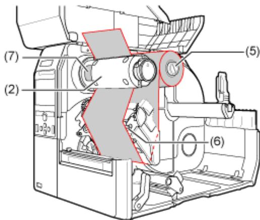
**6. Wind the ribbon counterclockwise to the ribbon rewind spindle (2) and grip sheet (7).**
