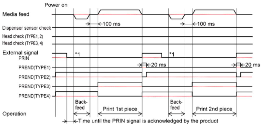
\*1 Keep the PRIN signal until the PREND signal is outputted.
