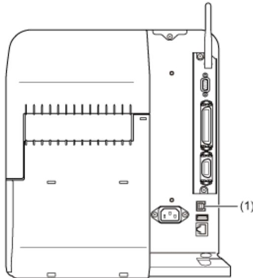
The USB interface is selected after connecting the USB cable to the computer and the product, and powering on the product while the computer is turned on.
