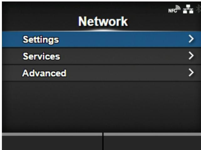
This menu is for using LAN and wireless LAN for the interface between the computer and the product.
