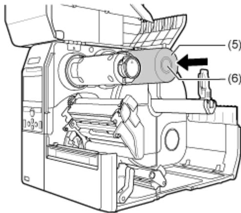
**8. From the ribbon supply spindle (6), pass the ribbon below the print head (7).**
