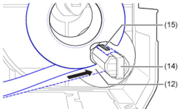
12. Rotate the liner rewriter (14) counterclockwise by hand, to wind the liner.
