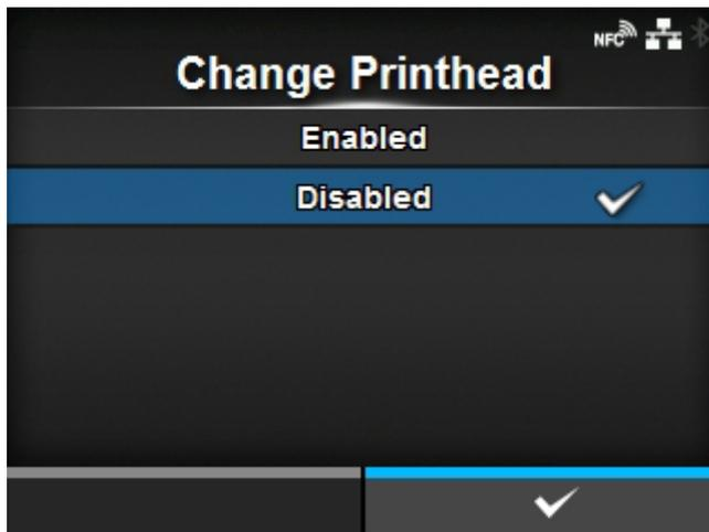
Enable or disable the notification function about when the print head needs to be replaced.
