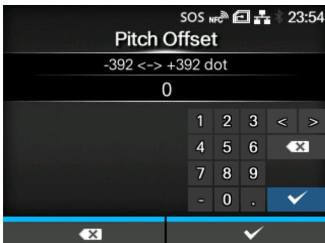
Pitch Offset adjusts the offset position and the pitch position at the same time.
