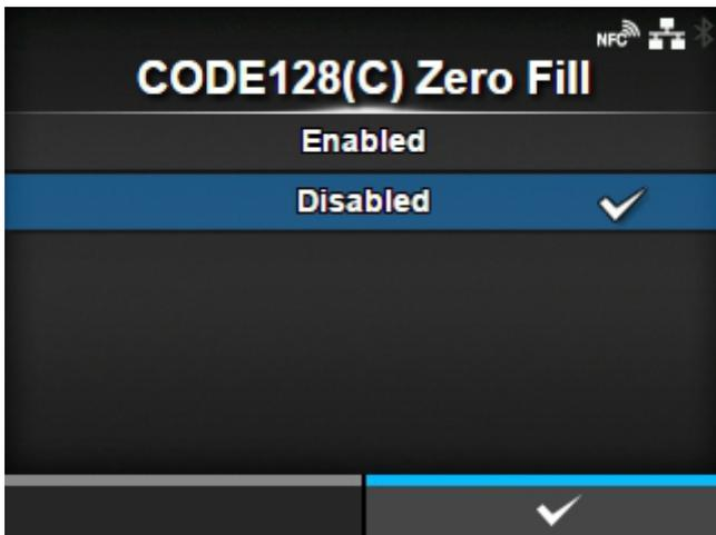
Set whether to allow odd digits and print the barcode with zero-filling at the end of the data when start code C is used in CODE128.
