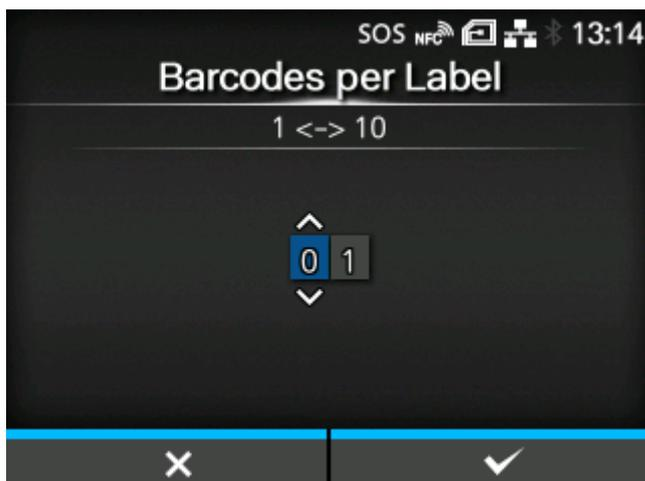
Specify the number of barcodes per label when you include barcodes which are not created by barcode commands as the target of the barcode readability check.
