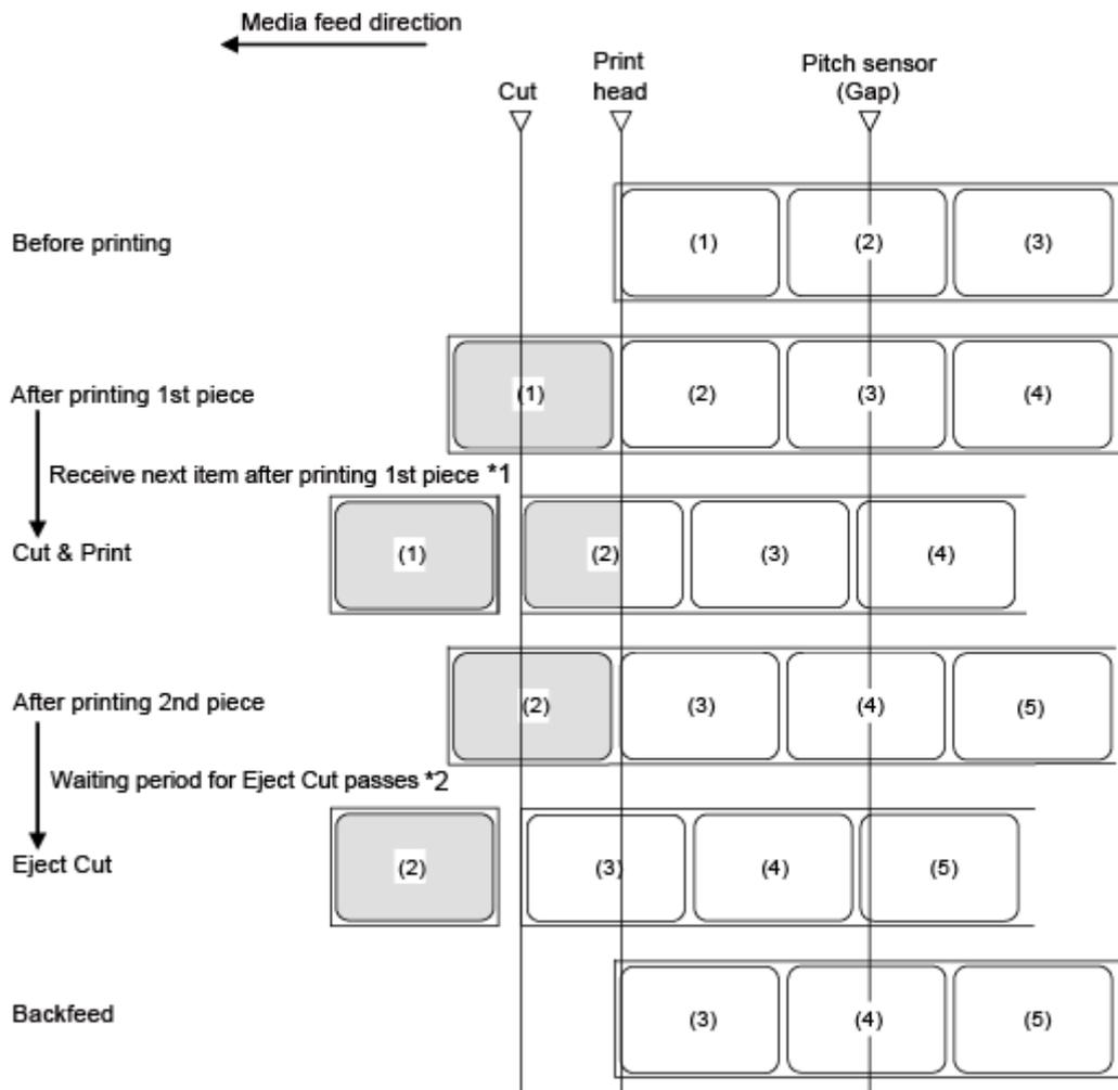
\*1 After printing, if the next data is received, printing will be done and the media will be cut on the cut position.
