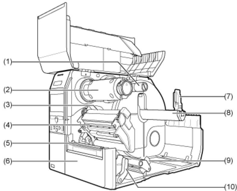
**(1) Ribbon supply spindle****(2) Ribbon rewind spindle****(3) Ribbon roller****(4) Print head (Consumables)**
