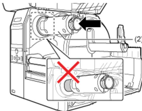
If there is any ribbon on the ribbon rewind spindle, remove it from the spindle before installing new ribbon.
