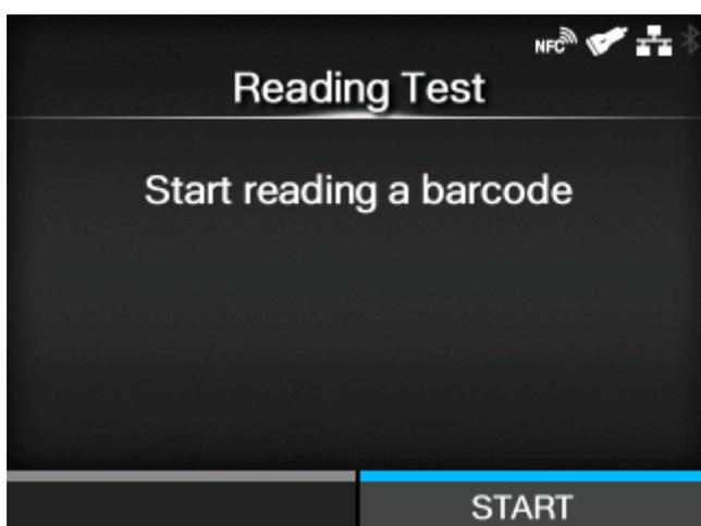
Perform a test read with the connected barcode checker.
