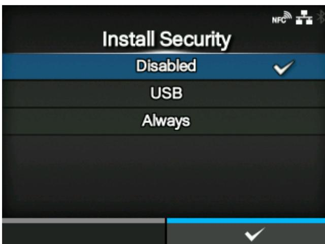
Enable or disable the password input for installing the pkg file to the product.
