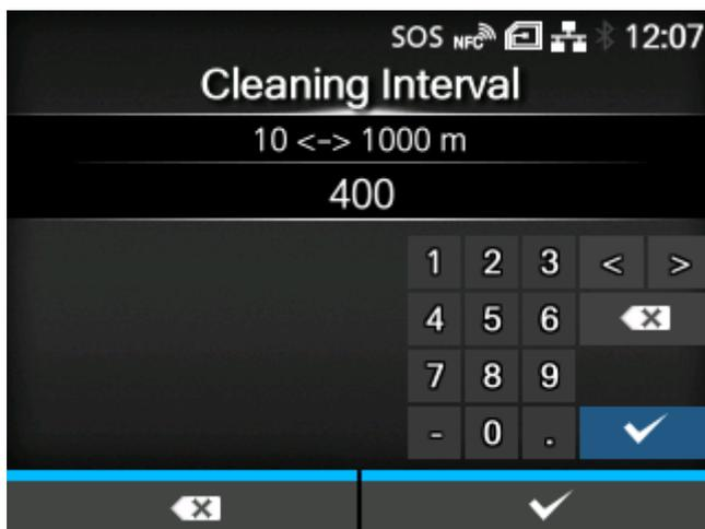
Set the notification interval about when the print head needs to be cleaned.
