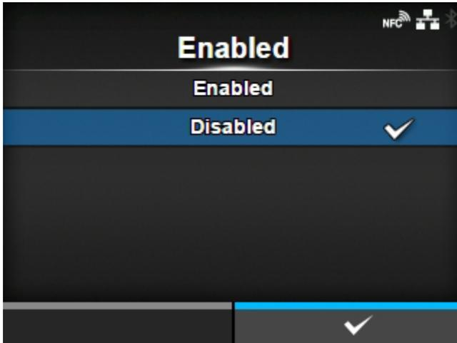
Enable or disable AEP (Application Enabled Printing) mode.
