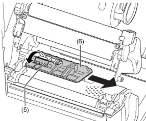
7. Clean the bottom of the media sensor guide using the cotton cloth dabbed with cleaning liquid.
