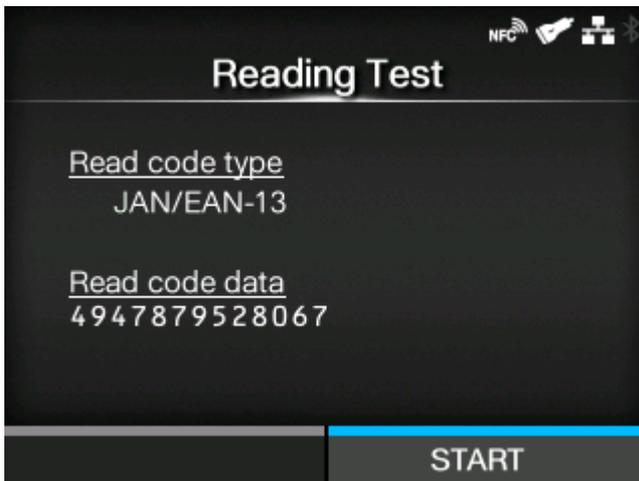
If reading is unsuccessful, or the displayed results of the read are not correct, adjust the position of the barcode checker by using the barcode checker stand. For details on how to use the barcode checker stand, refer to the Barcode Checker Stand Kit Installation Manual that came with the barcode checker stand kit.
