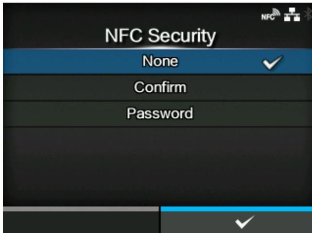
Set whether to show the confirmation message or enable the password input before settings are written to the product from an Android device with the NFC interface.
