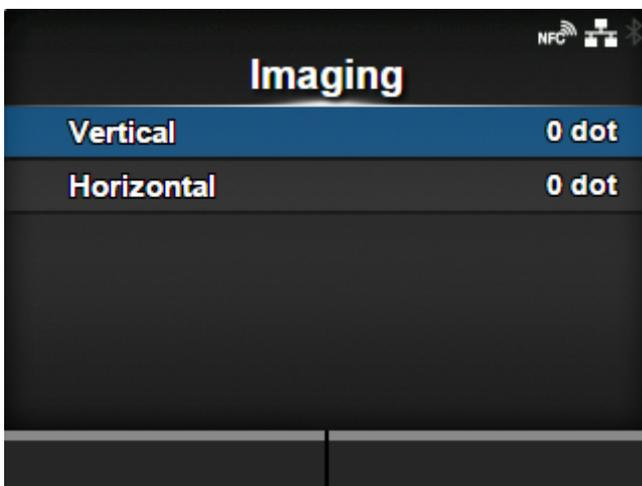
Set the print reference position in the vertical and horizontal directions.
