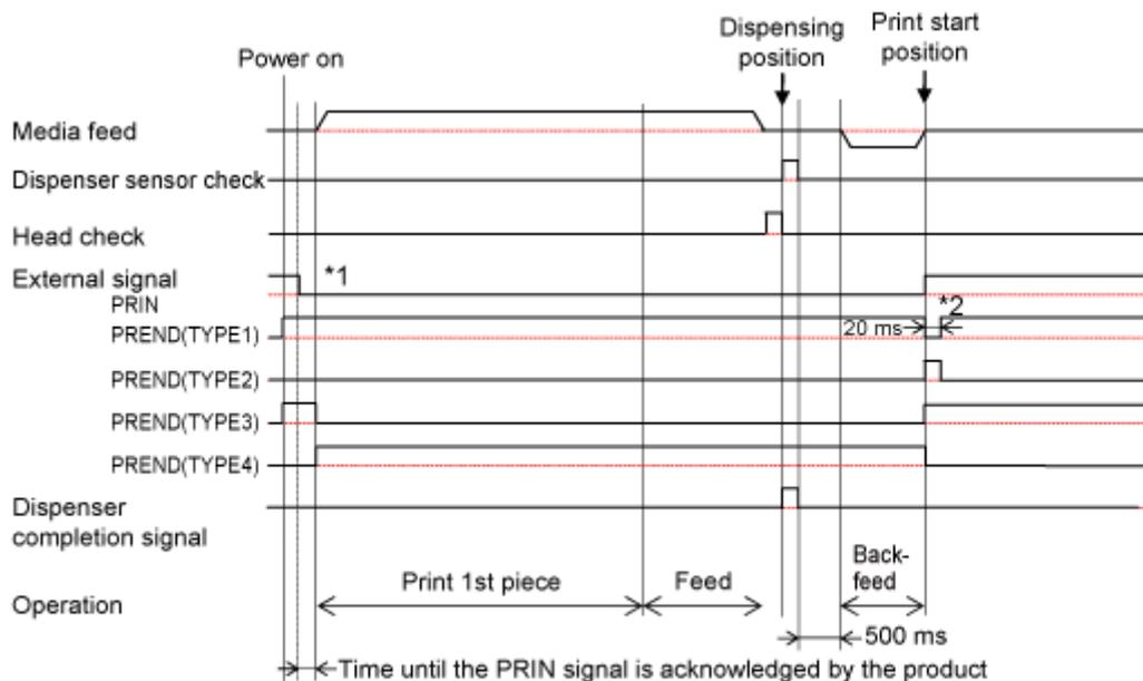
\*1 Keep the PRIN signal until the PREND signal is outputted.
