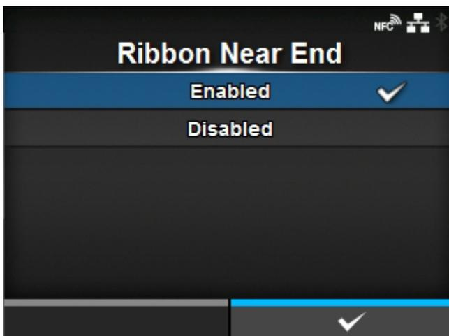
Shows or does not show the warning icon when the ribbon is about to run out. Printing does not stop even if the warning icon shows up.
