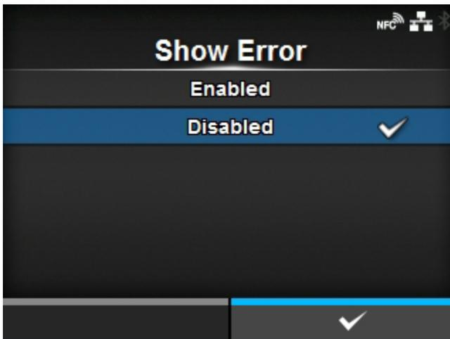
Enable or disable the command error indication when incorrect command or parameter is detected in the print data.
