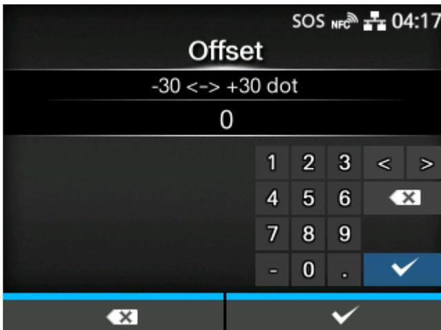
5. Change the setting value. Press the ◀/▶/▲/▼ buttons to select a number and then press the ← button to enter the number to the text box.
