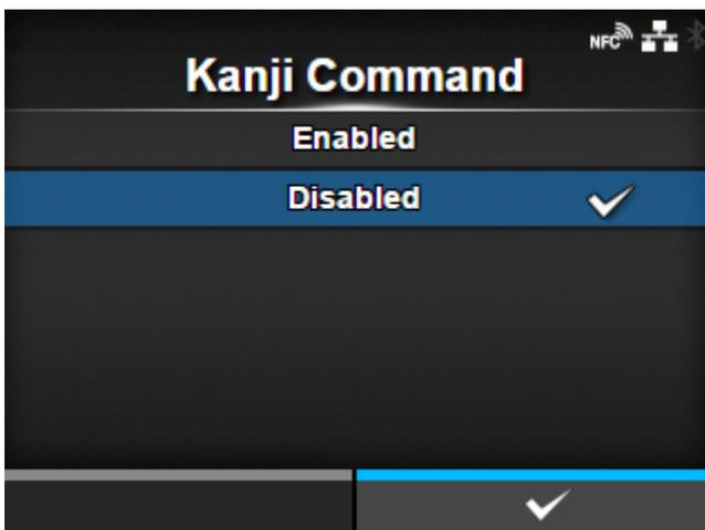
Set the product behavior when the received data includes the Kanji command ESC+K5, ESC+K6 or ESC+K7.
