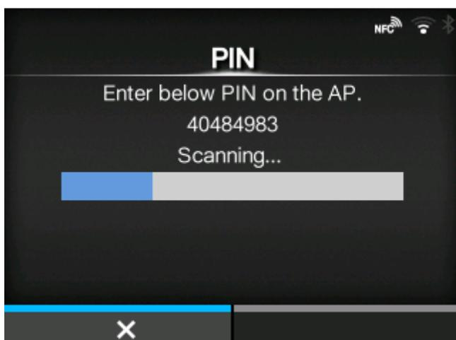
Set the wireless LAN connection using the PIN code method.
