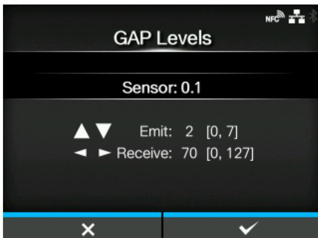
Manually set the Gap sensor level.
