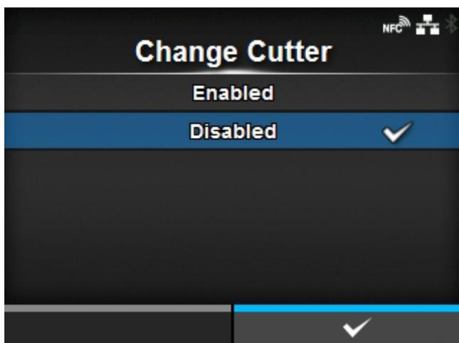
Enable or disable the notification function about when the cutter unit needs to be replaced.
