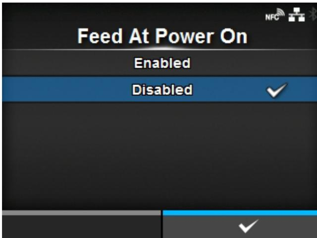
Set whether to automatically feed the media when the product is powered on.
