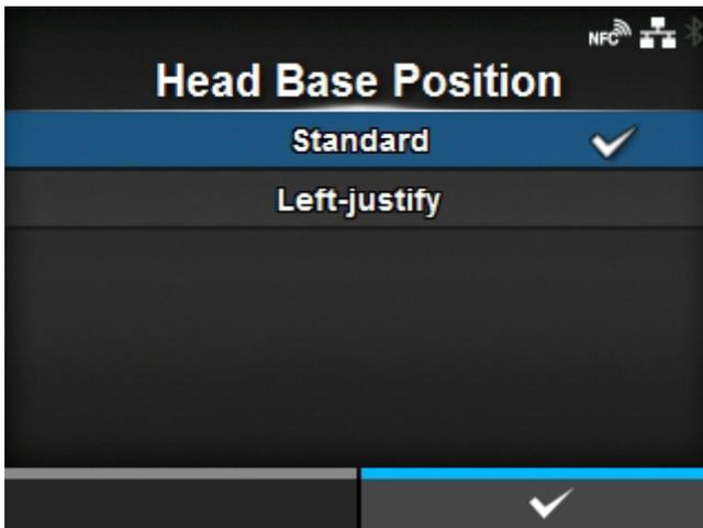
Set the position used for the base reference point for printing.
