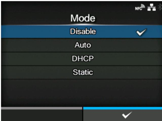
Select the IP address assignment method or disable IPv6.
