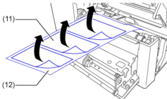
9. Pass the liner (12) through the gap of the dispenser unit to the inside of the product.
