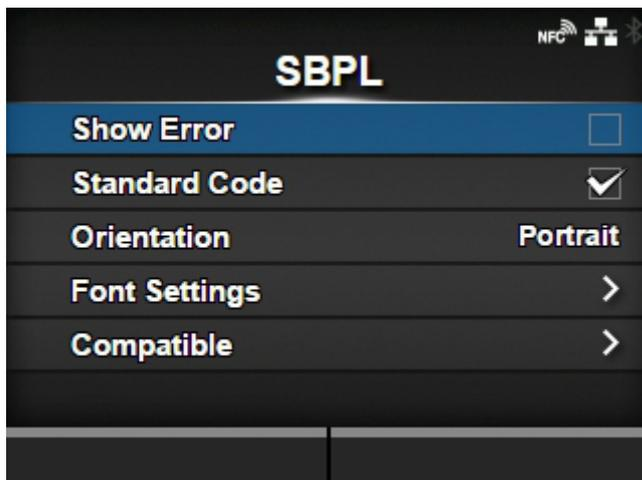
SBPL (SATO Barcode Printer Language) is the common command that controls SATO barcode label printers.
