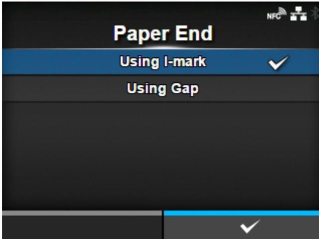
Select the sensor for sensing the paper end.
