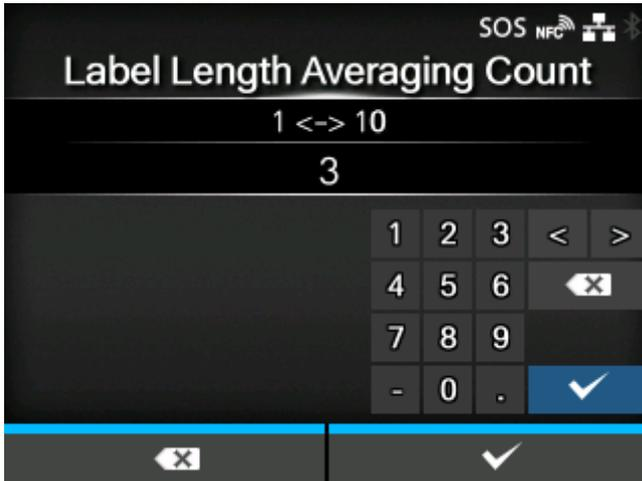
Set the number of labels measured to be used for averaging the automatically set label length when the [Micro Label Print Mode] is set to [Enabled] and the [Auto Label Length Detection] is set to [Enabled].
