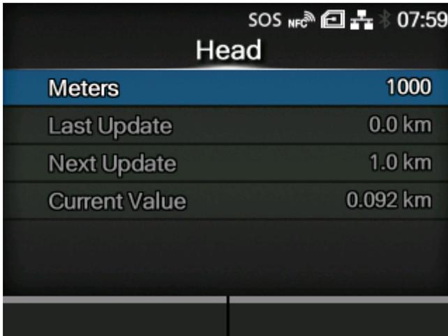
You can specify or check the print distance of the print head for the timing to perform the periodic notification.
