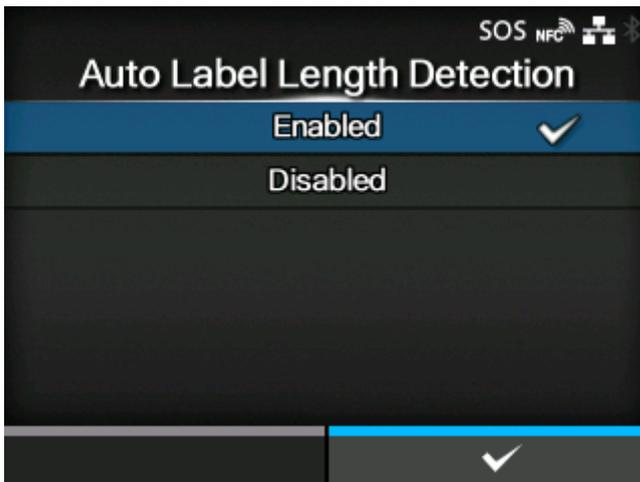
Enable or disable automatic measurement of label length when the [Micro Label Print Mode] is set to [Enabled].
