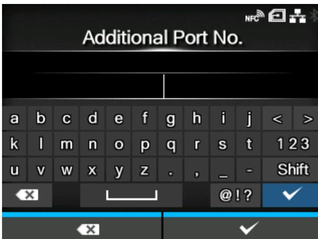
Register the TCP source port number to allow communication.
