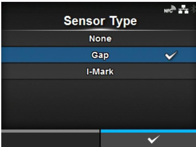
Set the sensor type for detecting the media.
