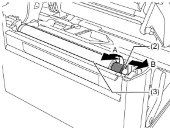
5. Install the new platen roller.
