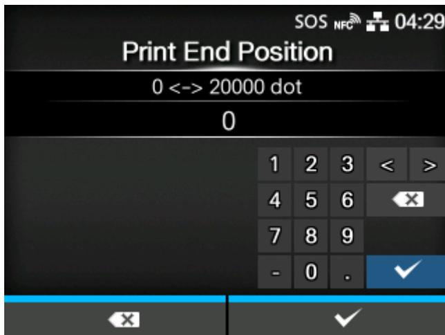
Adjust the media stop position or cut position when the [Sensor Type] is set to [None]. This adjustment also sets the blank amount from the media stop position.
