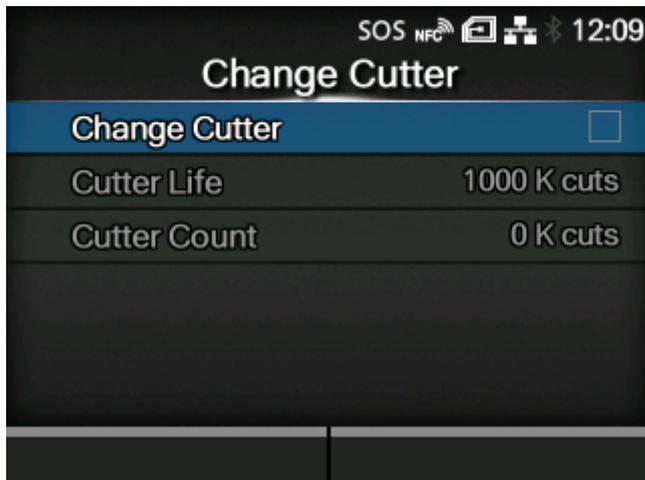
Notify when the cutter unit needs to be replaced.
