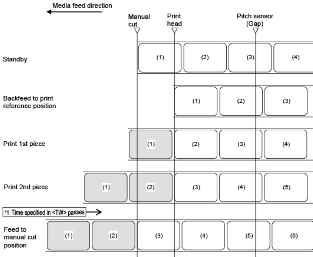
\*1 After printing, if the period specified in Option Waiting Time <TW> (initial value: 0 ms) has passed and if there is no print data remaining, the product will feed the media to the position for manual cutting.
