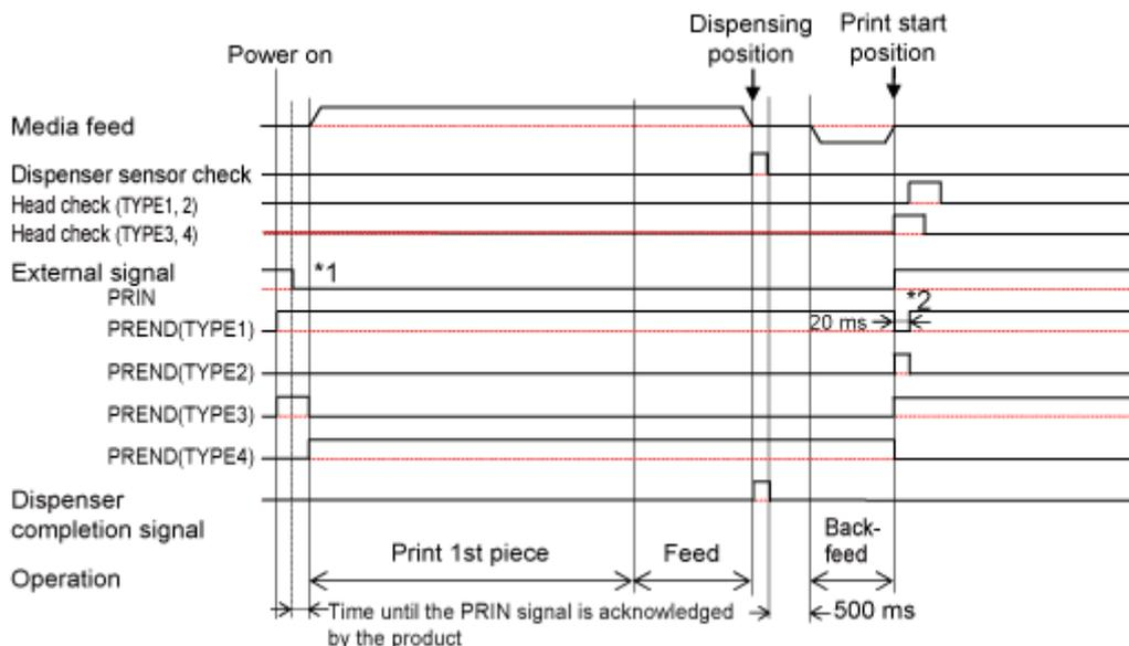
\*1 Keep the PRIN signal until the PREND signal is outputted.
