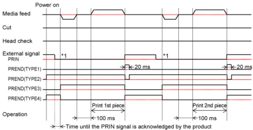
\*1 Keep the PRIN signal until the PREND signal is outputted.
