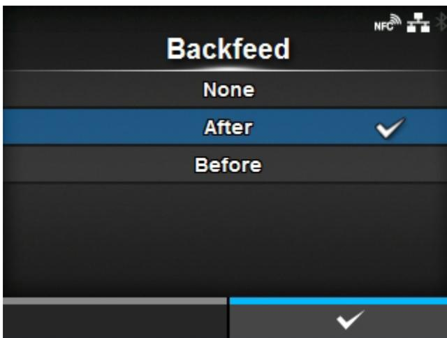
[Backfeed] is applicable when the print mode is set to tear-off mode, cutter mode, cut & print mode, dispenser mode or linerless mode.
