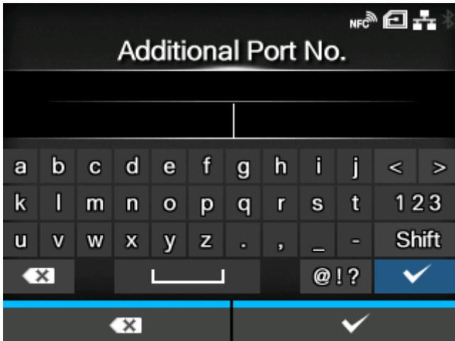
Register the TCP destination port number to allow communication.
