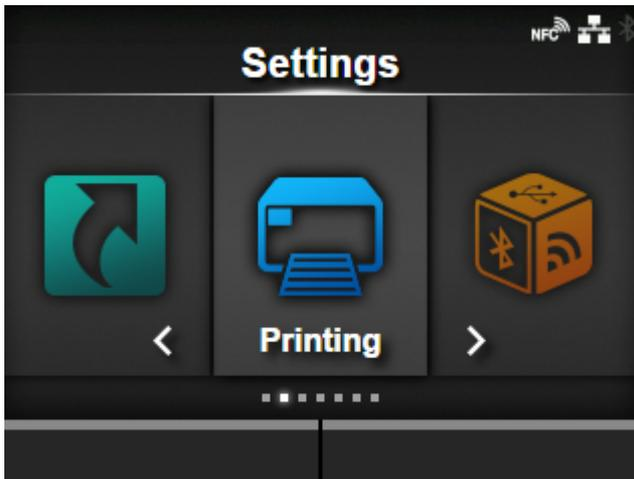
4. Press the ▲/▼ buttons to select [Speed], and then press the ⏪ button.
