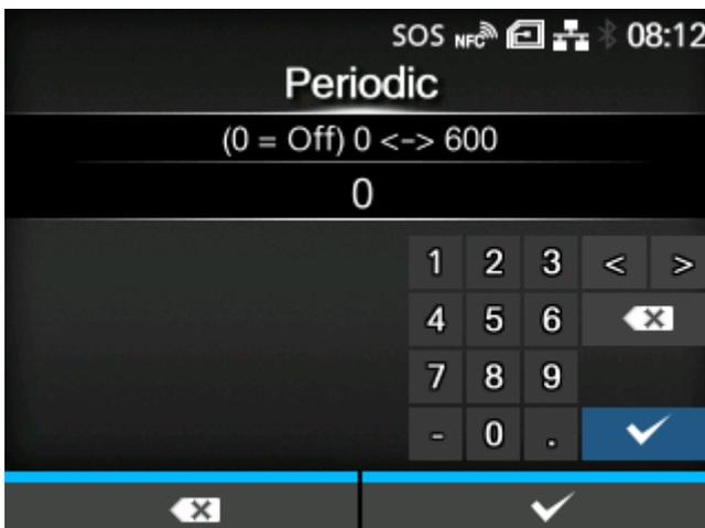
Set the interval of the ARP announcement in the range of 0 to 600 seconds.
