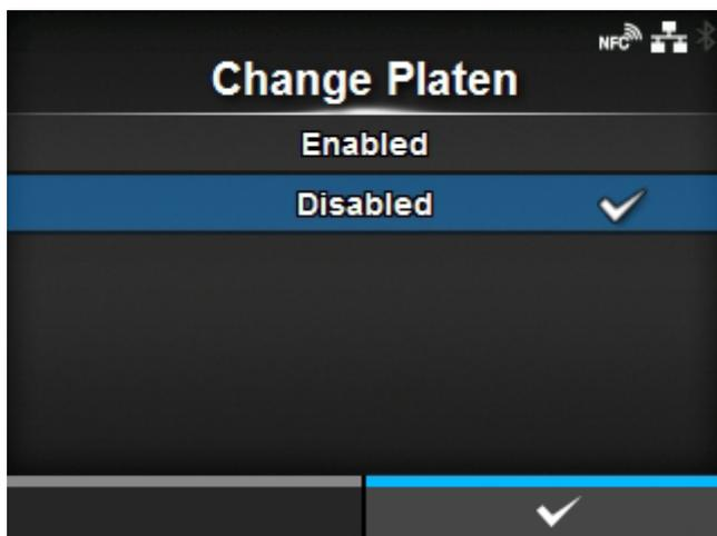
Enable or disable the notification function about when the platen roller needs to be replaced.
