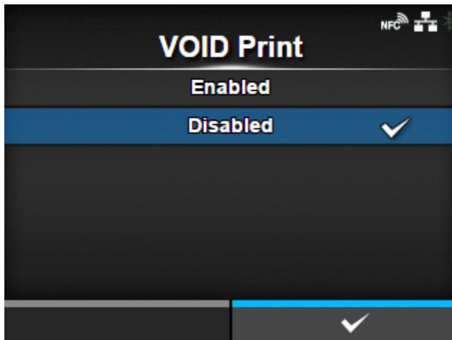
Set whether to print error marks on the media when a barcode reading error or barcode comparison error occurs.
