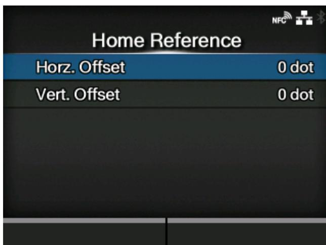
Adjust the print reference position by specifying the offset position in the horizontal and vertical directions.
