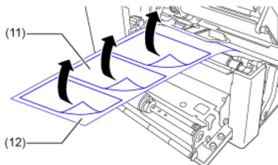
9. Pass the liner (12) through the gap of the dispenser unit to the outside of the product.
