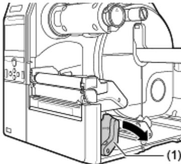
2. Press the print head down until the head lock lever is locked.
