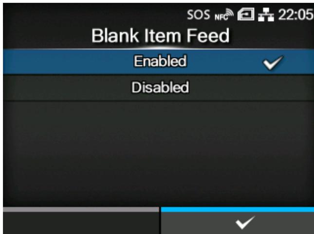
Set whether to feed a label with nothing printed on it when the product receives label formatting commands that do not generate any printable image.
