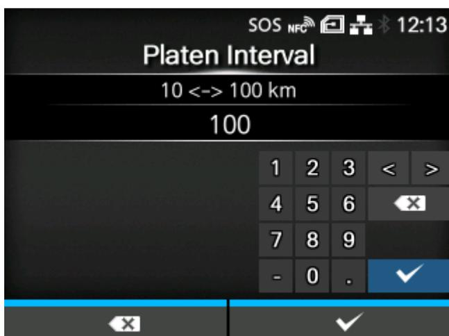
Set the notification interval about when the platen roller needs to be replaced.
