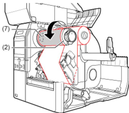
7. If the media is already loaded, press the print head down until the head lock lever is locked.
