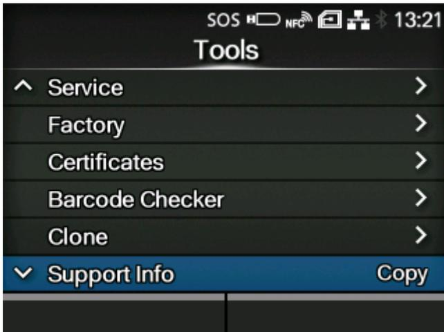
Save various information about the product, such as attached options, serial number, application versions and settings configuration, in a text file (.txt) to the USB memory.
