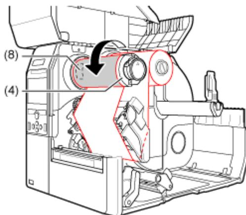
**10. Press the print head down until the head lock lever is locked.**
