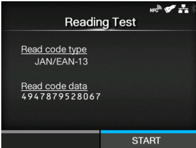
If the reading is unsuccessful, or if the displayed read result is not correct, adjust the position of the barcode checker by operating the barcode checker stand. For details on how to use the barcode checker stand, refer to the Barcode Checker Stand Kit Installation Manual that came with the barcode checker stand kit.
