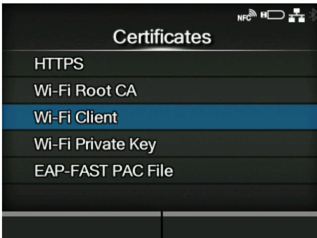
Install certificates used for Wi-Fi authentication and for HTTPS.
