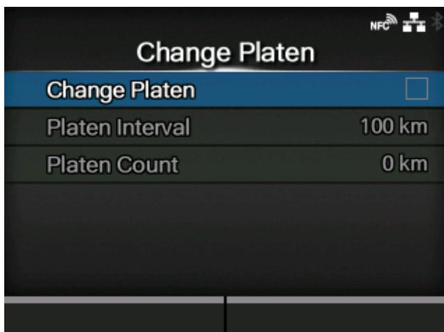
Notify when the platen roller needs to be replaced.
